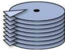
Figure 13: Platters in a HDD
