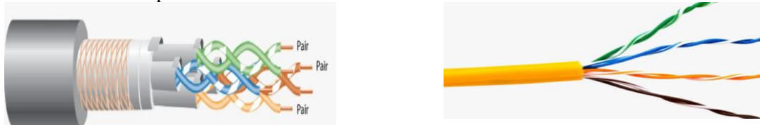
Figure 5.17: Shielded twisted pair and Unshielded twisted pair
