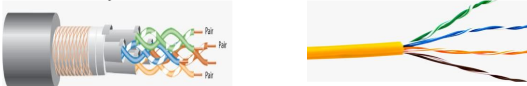
Figure 5.17: Shielded twisted pair and Unshielded twisted pair
